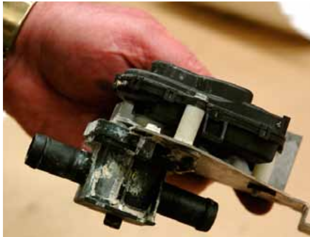
Debris can degrade seals and lead to a water valve failure. The white residue indicates a leak.
